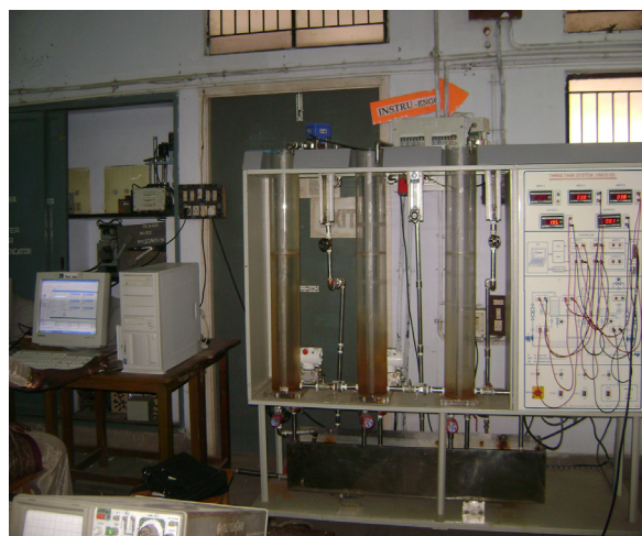
Fig. 1. Experimental Setup of Two Capacity Interacting Nonlinear Level Process.
