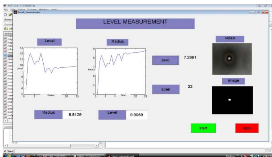
Fig. 3. Float-image level transmitter GUI.
