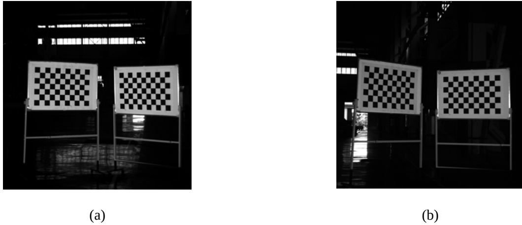
Fig. 5. Planar pattern boards for acquiring the point matches (a) left image (b) right image.
