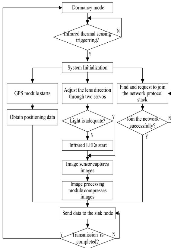
Fig. 5. Program flow chart of the wireless infrared image sensor node.
