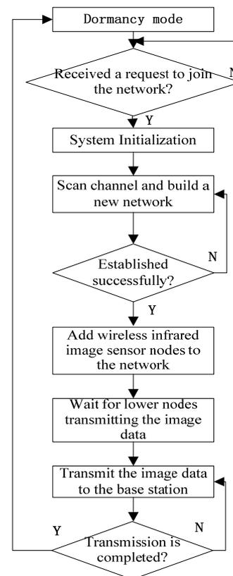
Fig. 6. Program flow chart of the sink node.
