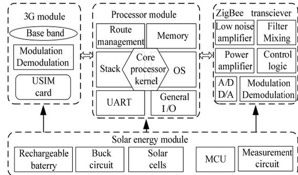
**Fig. 4.** Specific hardware architecture of the sink node.
