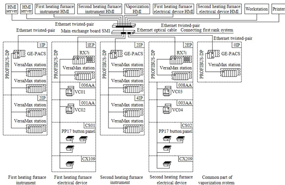
Fig. 6. The entire automation control system allocation picture of walking beam heating furnace.
