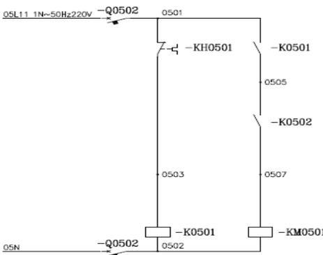
Fig. 10. The control circuit diagram of the first main pump of hydraulic station.
