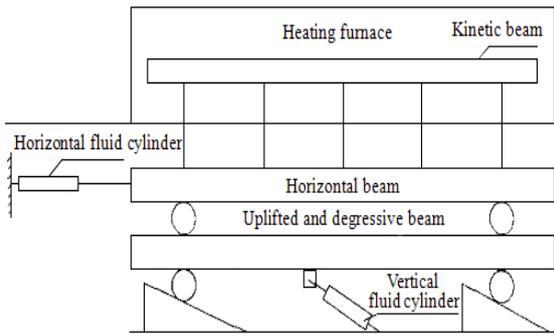
Fig. 9. Structure lateral picture of walking mechanism.
