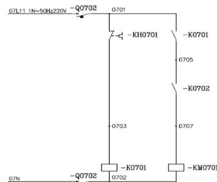
Fig. 12. The control circuit diagram of the third main pump of hydraulic station.
