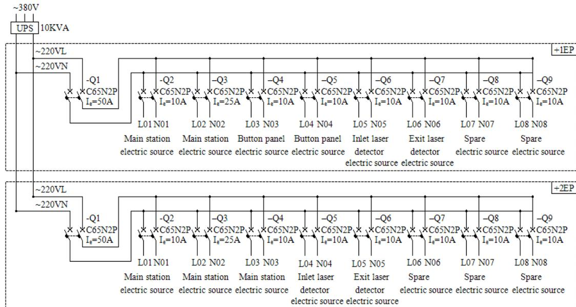
Fig. 7. The entire PLC power distribution system picture of walking beam heating furnace.
