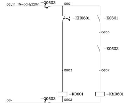
Fig. 11. The control circuit diagram of the second main pump of hydraulic station.
