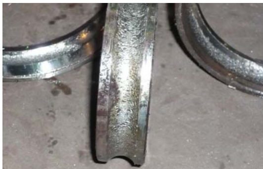
Fig. 12. Rolling bearing 3 with bad inner ring roller path abrasion.
