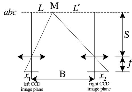
Fig. 1. Principle of parallel binocular CCD parallax ranging.
