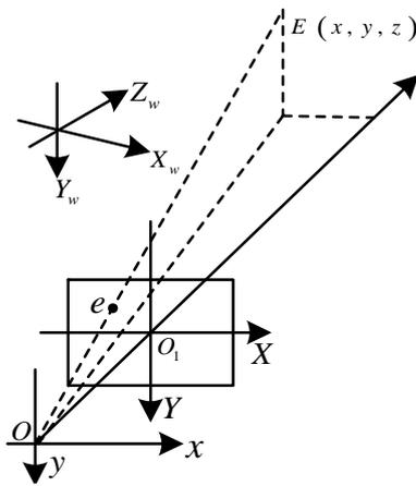
Fig. 2. The principle of pinhole imaging camera model.
