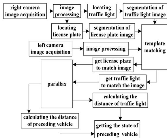
Fig. 6. The flow chart of the system of determining the movement state of preceding vehicles at traffic lights intersection.
