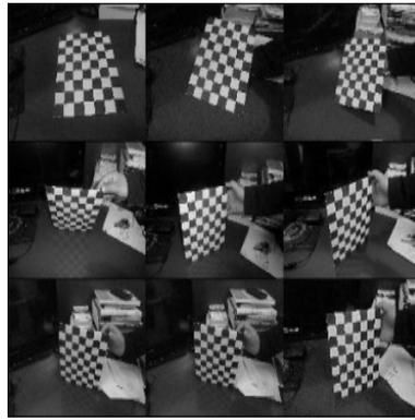
Fig. 4. Checkerboard calibration chart.
