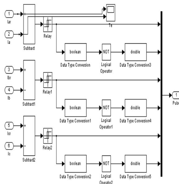
Fig. 6. Current control module.
