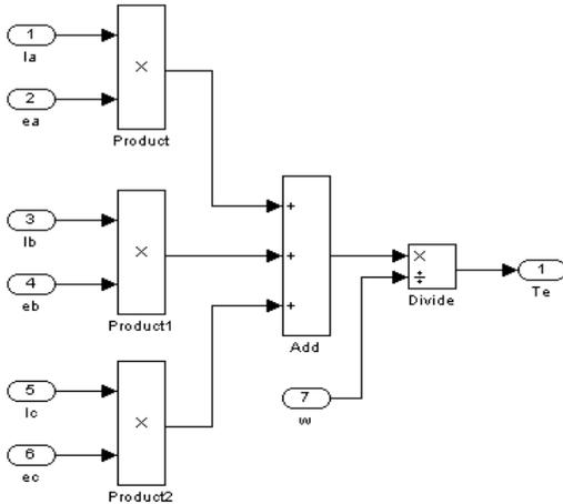
Fig. 3. Torque calculation module.
