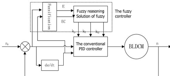
Fig. 7. BLDCM fuzzy PID control system structure.
