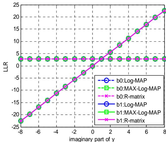
Fig. 3. The comparison of LLRs calculated by Log-MAP, MAX-Log-MAP and R-matrix for QPSK.
