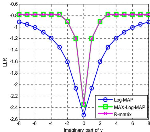
Fig. 4. The comparison of one bit soft value calculated by Log-MAP, MAX-Log-MAP and R-matrix for 16PSK.
