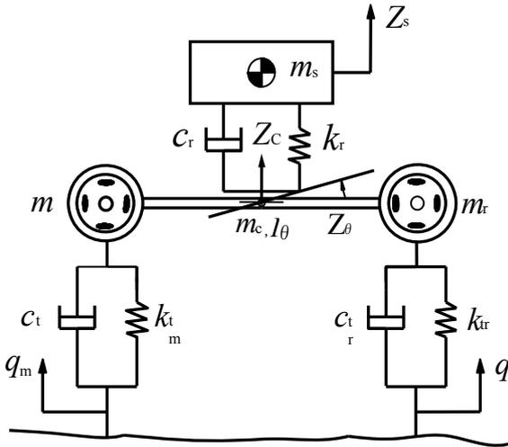
Fig. 2. Integral balanced suspension model considering rod moment of inertia.
