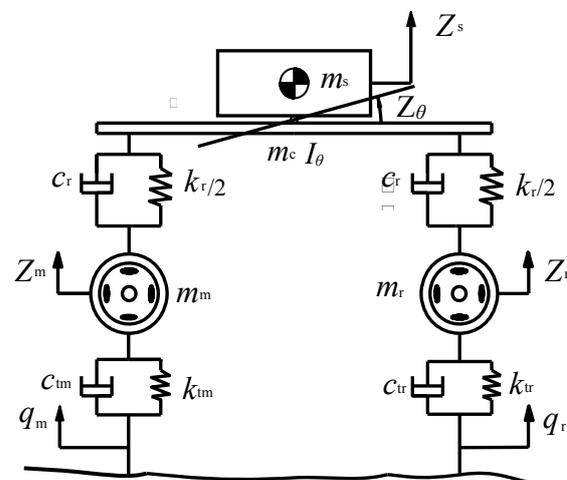
Fig. 1. Independent Balanced Suspension model considering rod moment of inertia.
