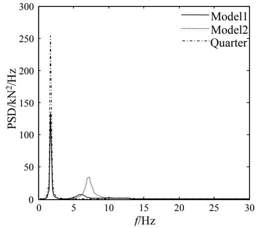
Fig. 4. PSD of tire dynamic force.
