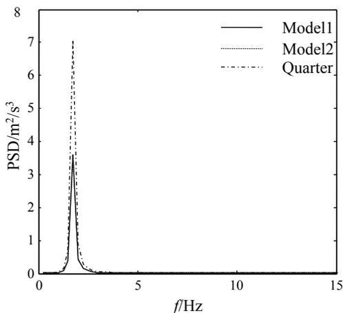
Fig. 3. PSD of sprung mass acceleration.
