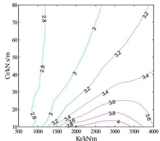
Fig. 14 (c). Contour pictures of road damage between suspension stiffness and damping parameters: C-class Road surface roughness.
