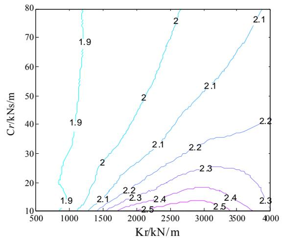
Fig. 14 (b). Contour pictures of road damage between suspension stiffness and damping parameters: B-class Road surface roughness.
