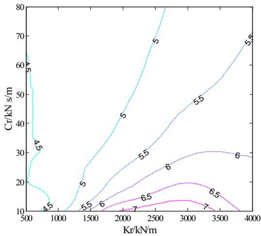
**Fig. 14 (d).** Contour pictures of road damage between suspension stiffness and damping parameters: D-class Road surface roughness
