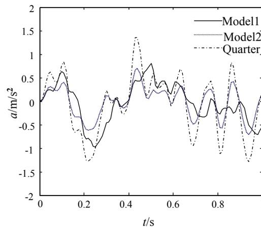
Fig. 5. Sprung mass acceleration response in time domain.
