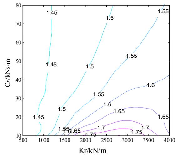
Fig. 14 (a). Contour pictures of road damage between suspension stiffness and damping parameters: A-class Road surface roughness.
