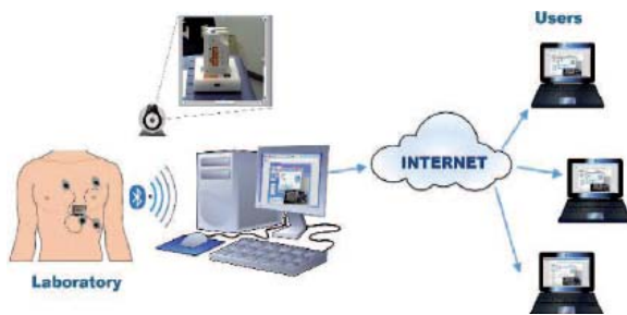
Fig. 11. General architecture of RePhyS.
