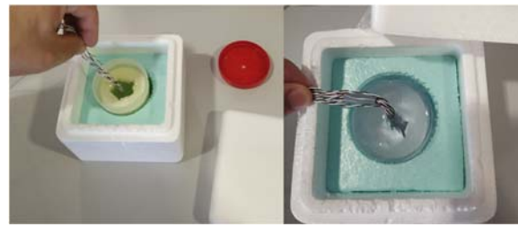
Fig. 5. The bundle of thermocouples under calibration is placed in the center of the calibration standard.
