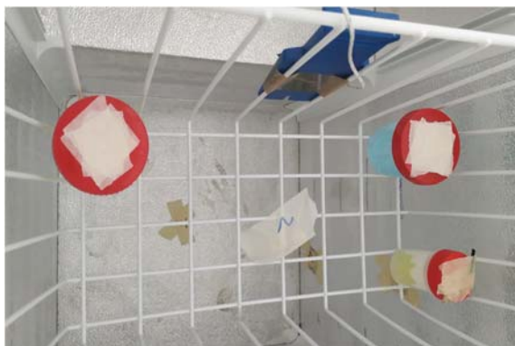
Fig. 4. The temperature standards are placed in a freezer chest.
