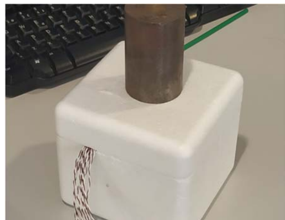
Fig. 6. The insulating enclosure is closed shut with the help of a weight on its lid, while the signals are acquired.
