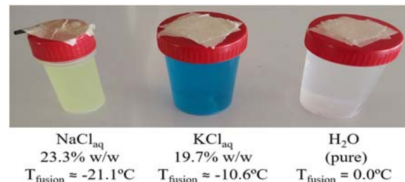
Fig. 2. The three temperature standards used in the thermocouple calibration.
