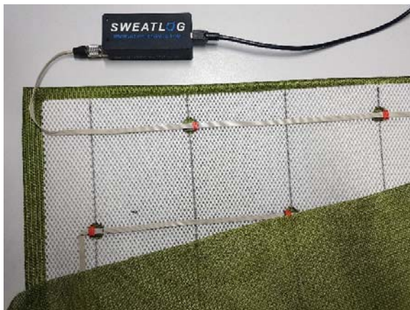
Fig. 8. SWEATlog logger and sensor array (mat) with up to 60 HIH8xxx sensors at one I2C ribbon (4 wires).
