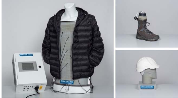
Fig. 5. SWEATOR torso with test jacket, SWEATOR foot and SWEATOR head with safety helmet.
