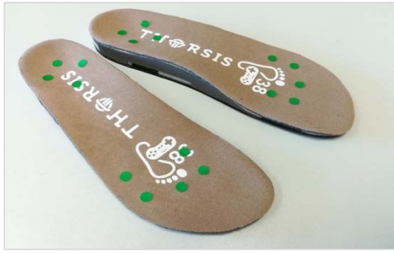
Fig. 5. Smart shoe insole with 3D-G sensors, pressure and temperature sensors indicated by green spots (Figure and device fabricated by Thorsis [21]).
