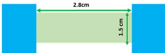
Fig. 4. Uniaxial tensile testing specimen.
