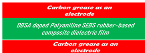
Fig. 2. Basic structure of stretchable carbon electrode-based ionic EAP strain sensor.
