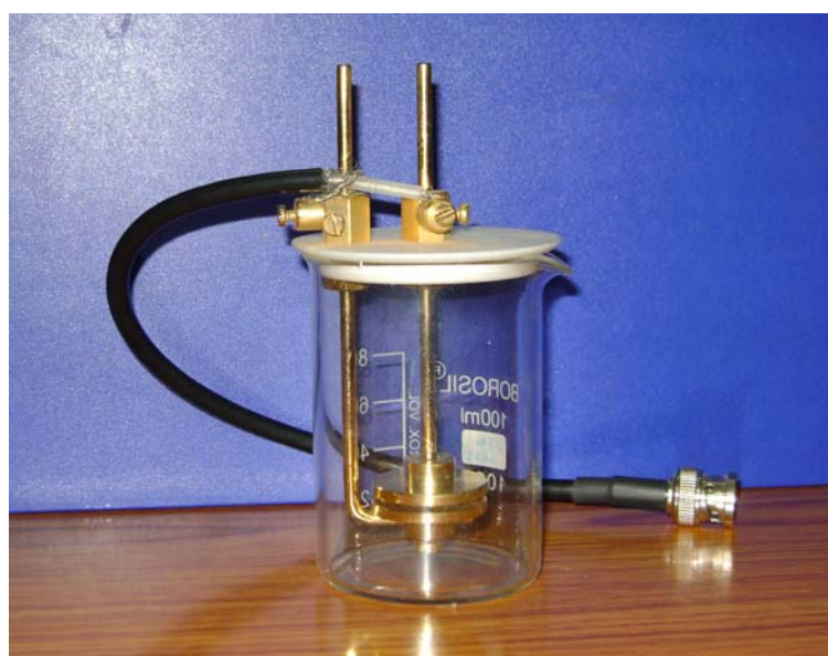
Fig. 1. Dielectric cell for an embedded based system for the measurement of dielectric constant spectroscopy for liquids.
