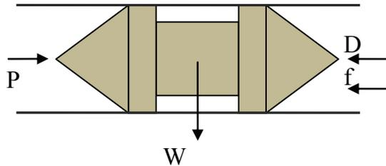
Fig. 4. Free body diagram of the MFL capsule.
