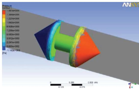
Fig. 8. Pressure distributions of the module in 3D view.
