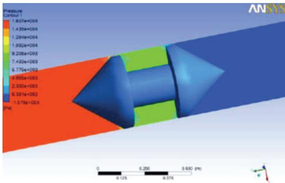
Fig. 5. Pressure distribution exists on the developed capsule.
