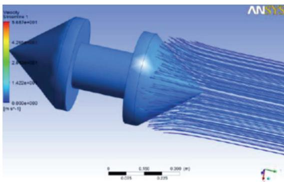
Fig. 6. Steamline simulation result of the developed capsule.
