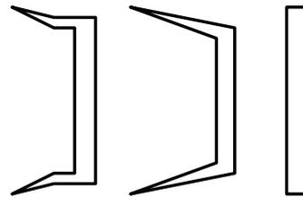
Fig. 1. Types of seal element used in PIGs.
