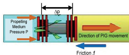
Fig. 2. Movement mechanisms inside a pipeline of a PIG
