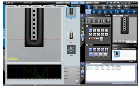
Fig. 6. Photomicrograph of release holes in the beam of the Fuze G-Switch.
