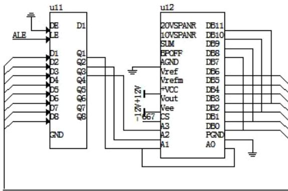
Fig. 5. AD667 hardware connection diagram.
