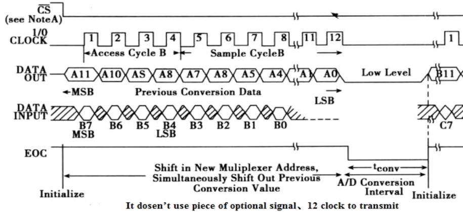
Fig. 3. TLC 2543 timing program diagram.
