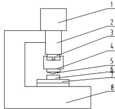
Fig. 2. Loading system organization diagram.
