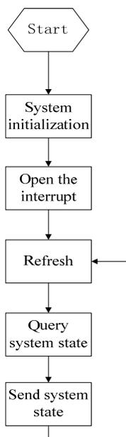
Fig. 6. The process of serial port interrupt program.
