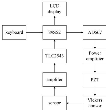
Fig. 1. Principle diagram of the control system.
