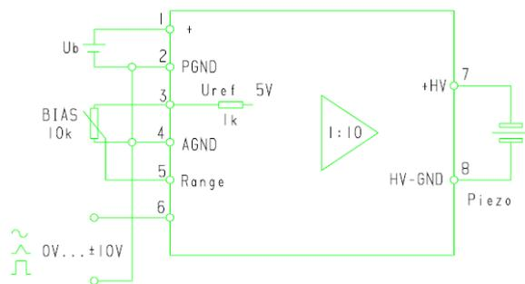
Fig. 4. Amplify circuit of E-660.
