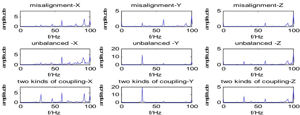
Fig. 3. Frequency domain characteristic figure of the rotor with faults.
