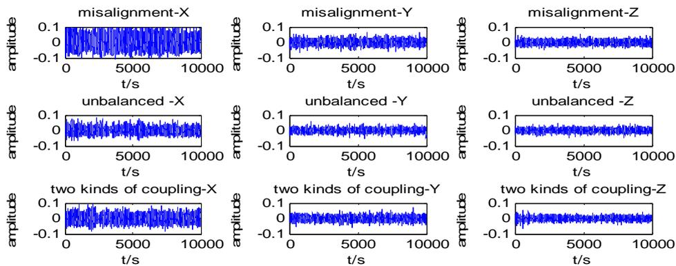
Fig. 2. Time domain characteristic figure of the rotor.
