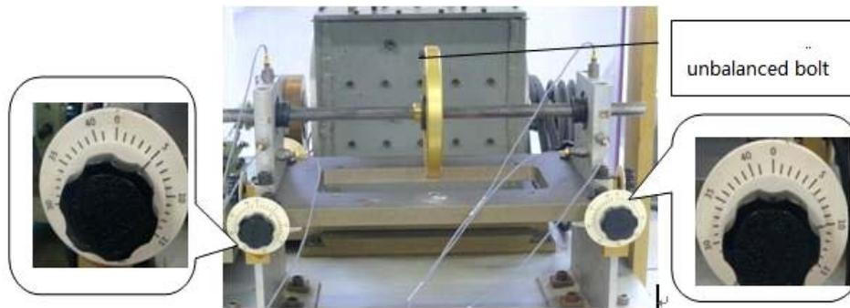
Fig. 1. Fault simulation of imbalance and misalignment in rotor system.
