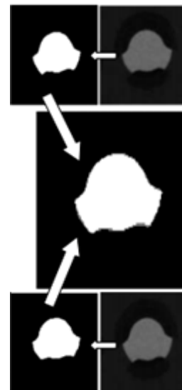
Fig. 3. Defect detection scheme by image subtraction.
