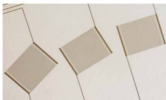
Fig. 4. Interdigitated capacitors built on glass substrate with gold fingers.
