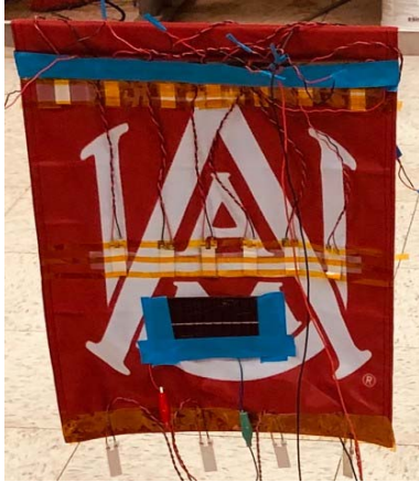
Fig. 1. An inverted flag with a mini flexible solar panel and piezoelectric/pyroelectric transducer strips.
