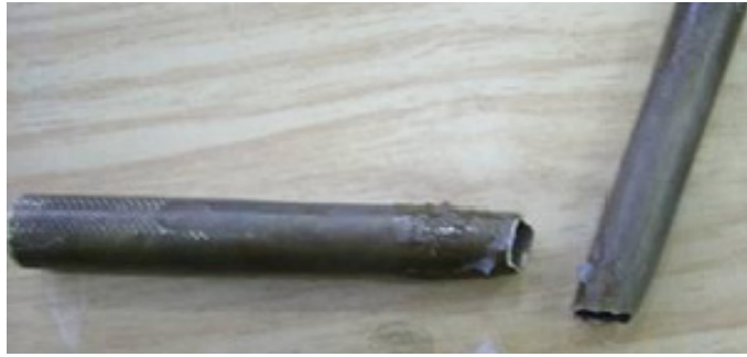
Fig. 9. Brass pipe after stretch cracking ( \phi 10 \times 150 mm and 0.5 mm thickness).
