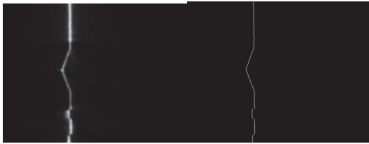
Fig. 5. Gaussian Blur and subpixel center line.
