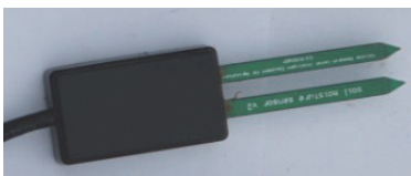
Fig. 2. Structure profile of soil moisture sensor.
