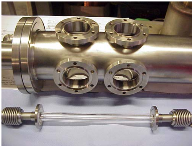
Fig. 1. Test rig for optical and capacitive measurements (prior to assembly): The conveyor pipe (bottom) comprises a quartz glass section of 230 mm length and two mechanical axial compensation modules to minimize the mechanical stress inside the glass section. For thermal insulation reasons, the conveyor pipe is inserted into stainless steel tubing (top) that is evacuated when operating the sensor. The outer tubing holds flanges for optical windows and electrical connectors.
