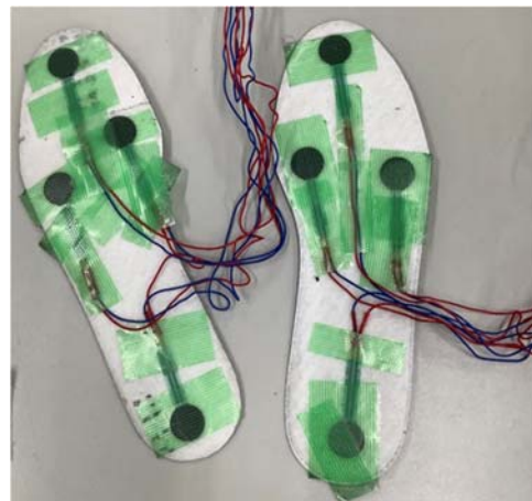
Fig. 1. Prototype insole sensor (bottom surface).
