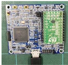
Fig. 1. MK109V3 connected to a PC through a USB cable.
