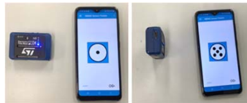
Fig. 20. Example indication of which side is facing up.
