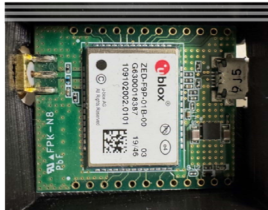
Fig. 4. RTK-GNSS receiver module (u-blox ZED-F9P) used for ground-truth position measurement in the field experiments.
