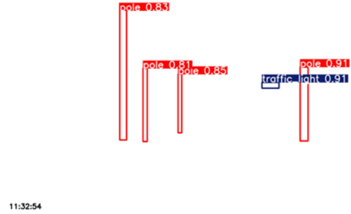
Fig. 9a. YOLO detected bounding box only image of the start point of the evaluation course. The second trip at 11:32:54.
